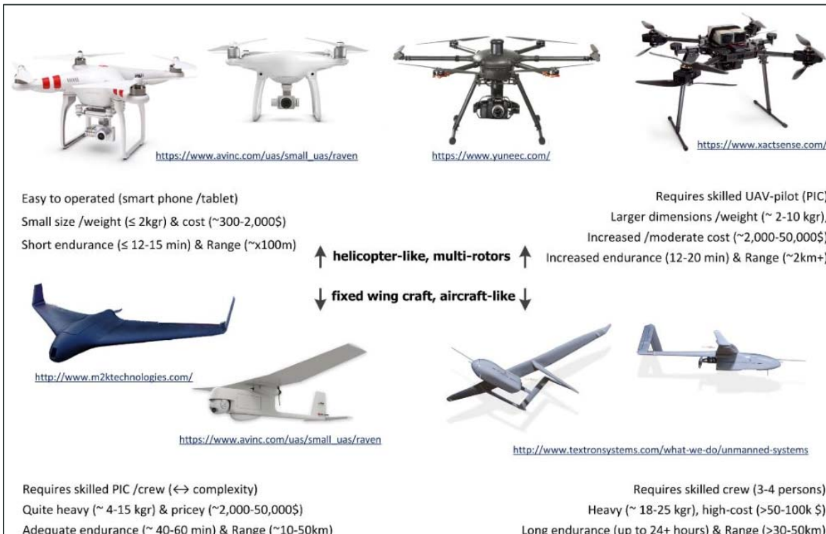
Figure 3 Drone size examples (Ntalakas et al. 2017).
