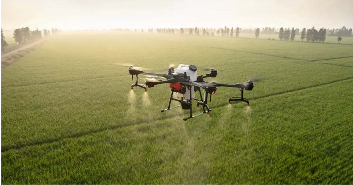
Figure 8 Example of drone spraying apparatus (equinoxdrones.com).
