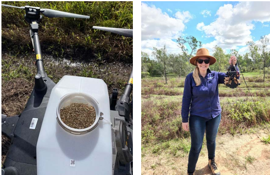
Figure 10 Examples of seed payload (left), and a modified claw attachment (right) supplied by provider as a solution to disperse uniquely shaped seeds from the case study.
