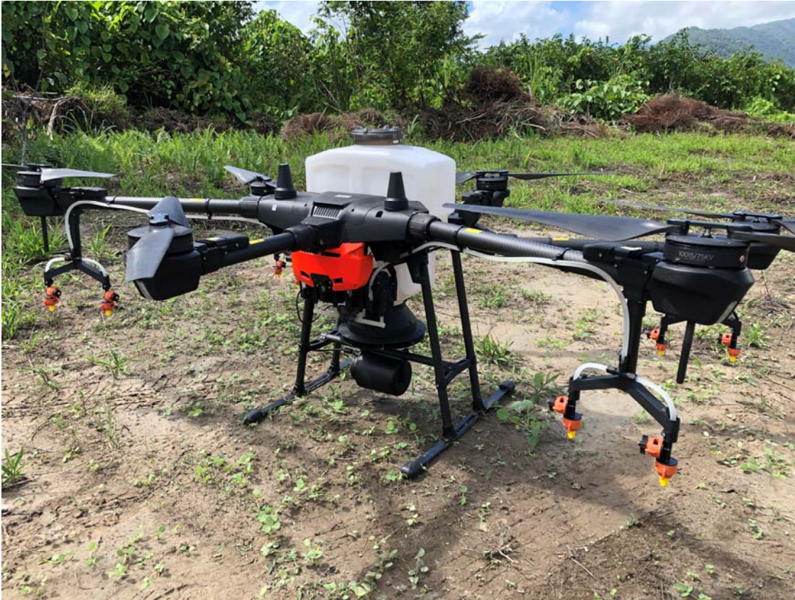
Figure 5 A larger drone used to distribute herbicide for weed treatment in the case study (photo credit: Marcus Bulstrode, DAF).
