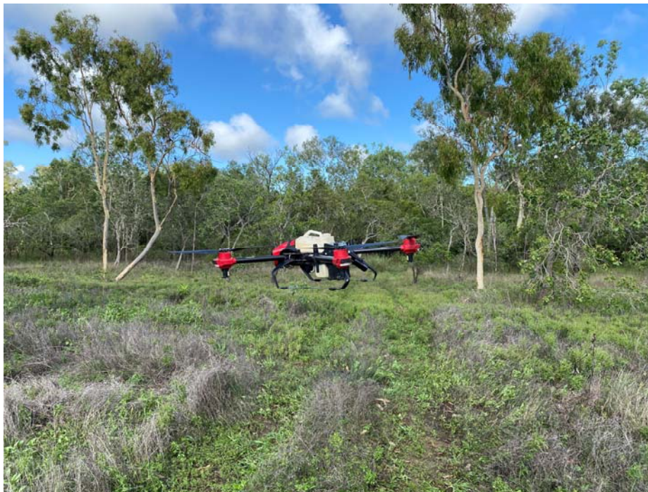
Figure 9: Example of a spraying drone used in the case study.
